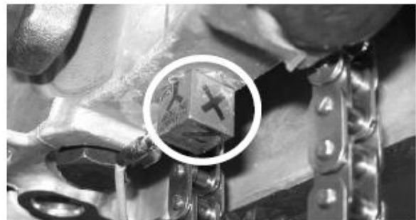
Triaxial accelerometer at crankshaft bearing
